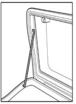
**Note:** Only the bottom "L" end of the stay needs to be removed for the lid to close; the top portion of the lid stay can remain installed.
